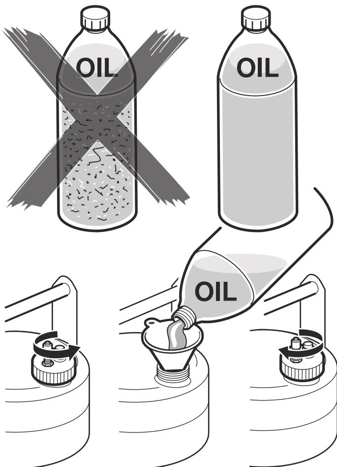
**en** Fill the fuel tank with filtered plant oil.
