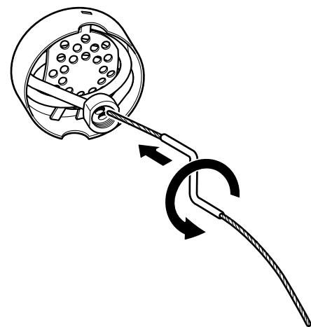
**en** Remove deposits in the evaporator with the short side of the S-shaped cleaner. Tap the residues out of the evaporator.
