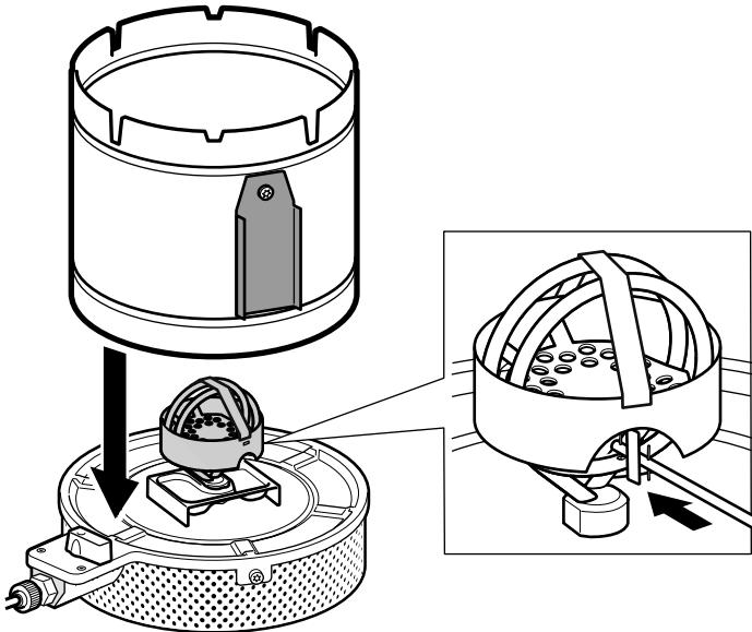
**en** Fit the wind protector in place. Ensure the flap is in a suitable position for nozzle cleaning.
