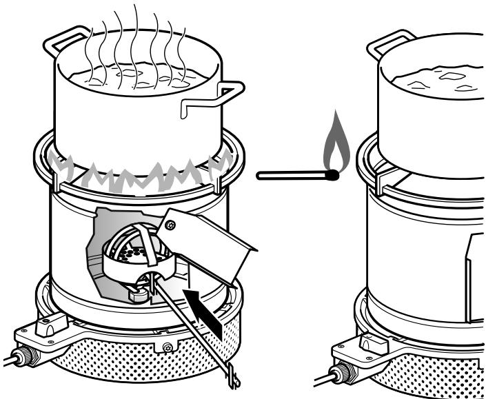
**en** If the flame is uneven, the nozzle must be cleaned during operation. To do this, clean the nozzle through the flap opening with the nozzle cleaner. If necessary, relight the flame.
