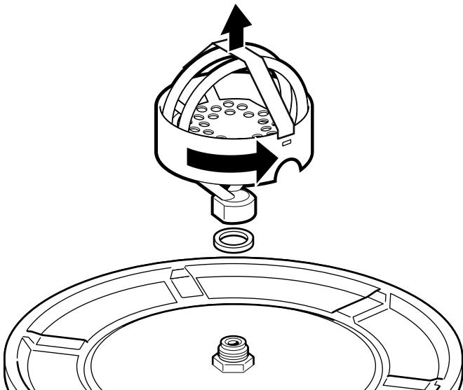
**en** After it has cooled down, unscrew the evaporator.
