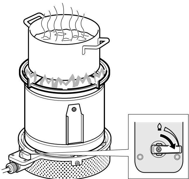
**en** To switch the stove off, close the rotary knob.
