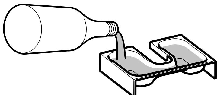
**en** Fill the preheating bowl up to the mark with alcohol. (Alcohol content at least 90%)
