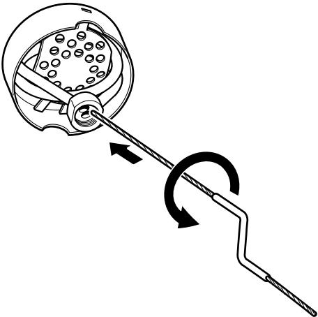
**en** Remove deposits in the evaporator with the long side of the S-shaped cleaner. Tap the residues out of the evaporator.
