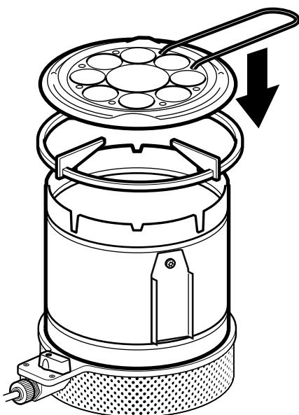
**en** Place the pot carrier and simmer plate onto the wind protector.
