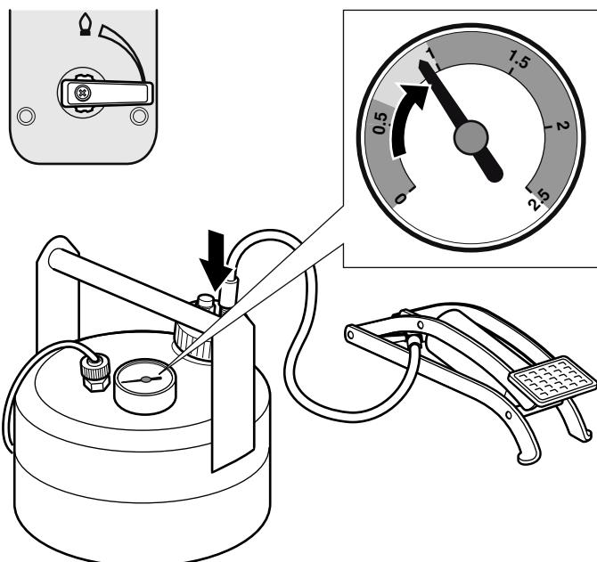
**en** The rotary knob must be closed. Build up pressure in the fuel tank using the pump until the pressure gauge reaches the end of the green zone (1 bar).
