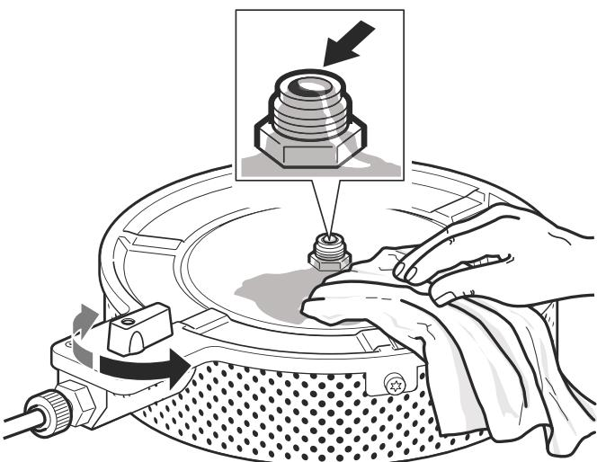
**en** Briefly open the rotary knob until oil emerges. Remove oil residue from the base plate.
