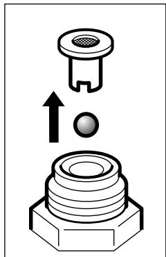
**en** Remove the filter and ball and clean. Take care not to lose any small parts.
