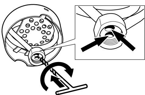
**en** Remove deposits in the evaporator first with a drill. Tap the residues out of the evaporator.
