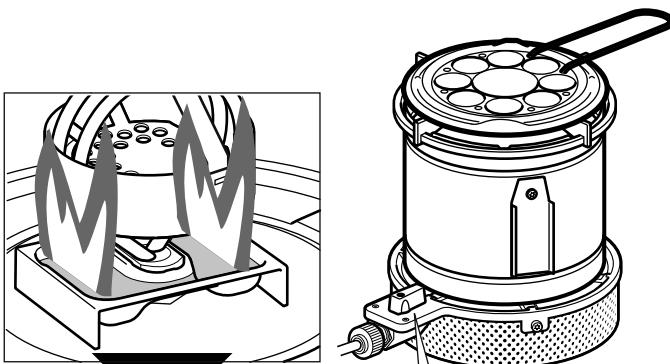
**en** Open the rotary knob after the first flame is extinguished. The ignition temperature has now been reached.
