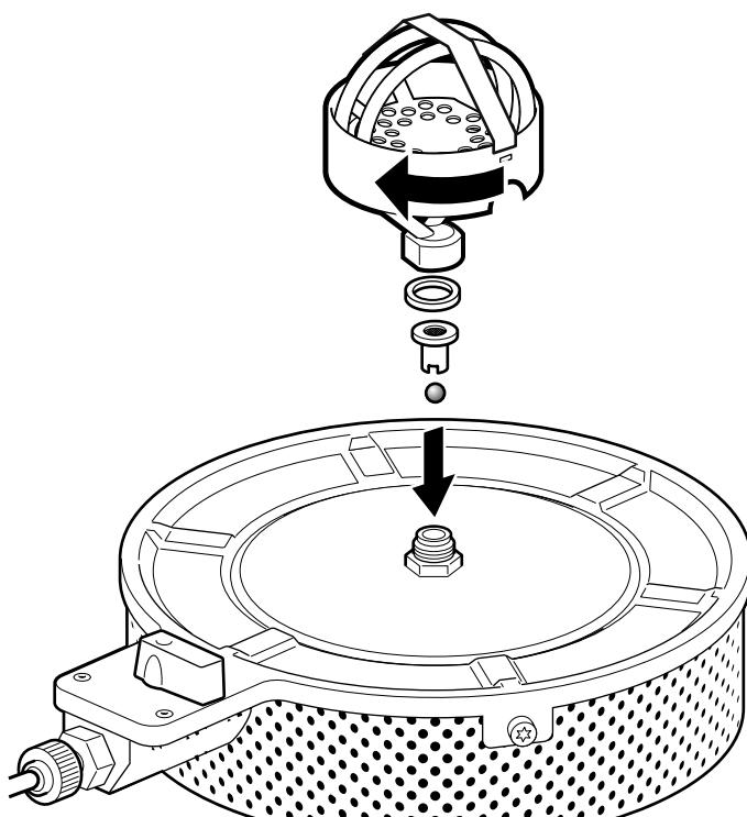
**en** Insert ball and filter, and place the seal in position. Screw on the evaporator and firmly tighten.
